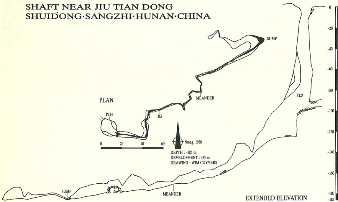
Fig. 14. Shaft near Jiu Tian Dong, PLAN AND EXTENDED SECTION.
