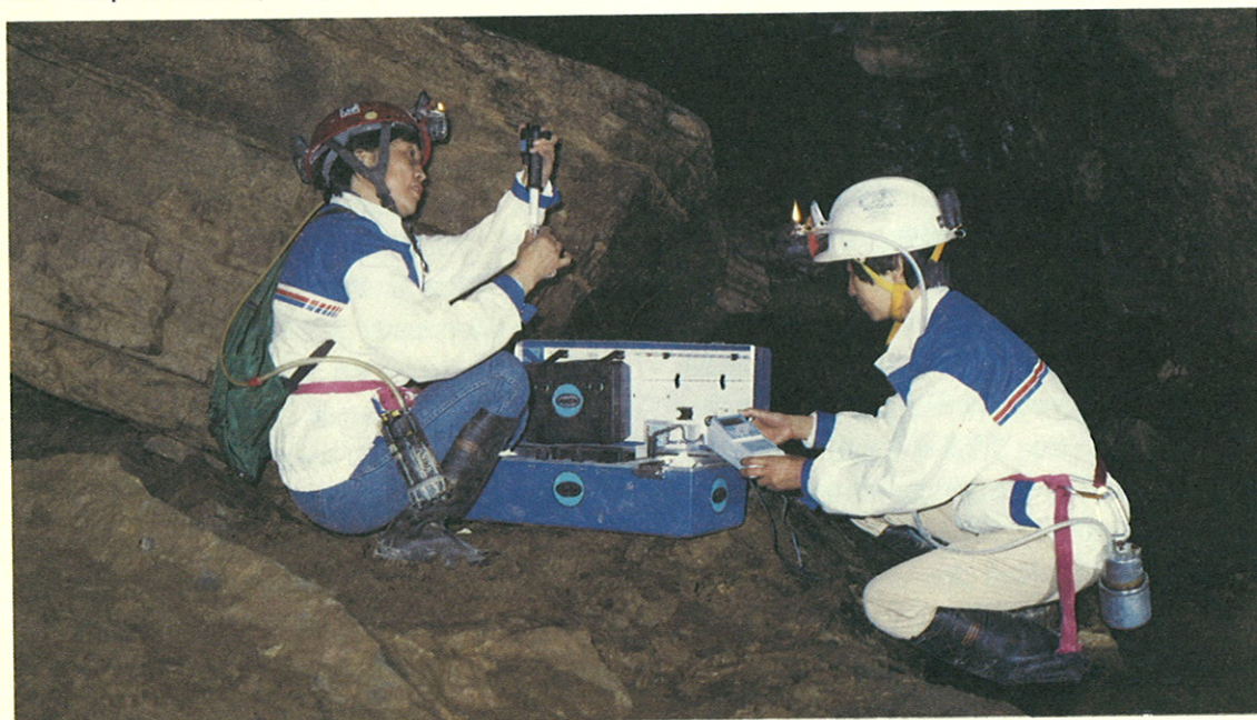
Hach Drel/5 portable laboratory in Cold Wind Cave.
